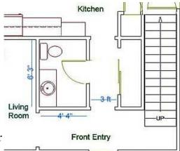
Simply widening the doorway wouldn't do the job. So we W-I-D-E-N-E-D it to 72" to accommodate double doors. Regular doors would be in the way of driving the wheelchair in. The key to success was using 2 two bifold doors. Instead
