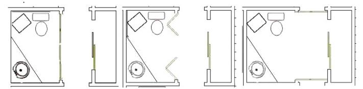
Since we have a basement under the bathroom it was quite easy to move the toilet about a foot away from it's original position. This allowed my wheelchair to be along side the toilet for transfers. Removing the vanity and putting the sink in a corner mounted counter top made it possible for me to roll under the sink for shampooing, etc. Even though I am now on a vent, I can still lean forward over the sink.
